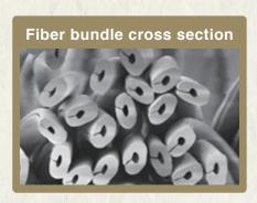
\*Flat C cross-sectional shape keeps functional agent within hollow structure for advanced functionality.
